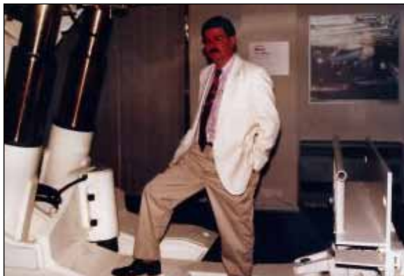
Ted Latusek examines the hydraulic roof support — designed to prevent a cave-in on a longwall section — at a plant in England in 1993.
